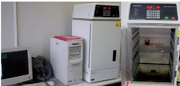
**Figure 1.** Faxitron M20 digital radiography system
